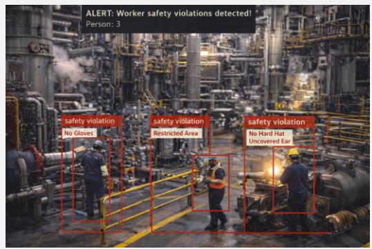
Example of computer vision detection of safety violations at a refinery
